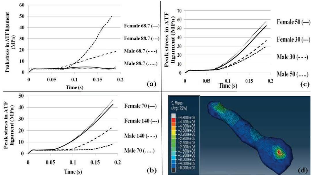
**Figure 5.** Diagram of peak stress in ATF ligament under 2 different conditions for males and females in : (a) First strategy (b) Second strategy (c) Third strategy; (d) Stress distribution pattern in ATF ligament in females, initial angle of ankle with ground = 68.7.
