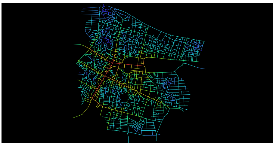
Figure 2: Analysis of the site's access to the Lahijan city using space syntax
